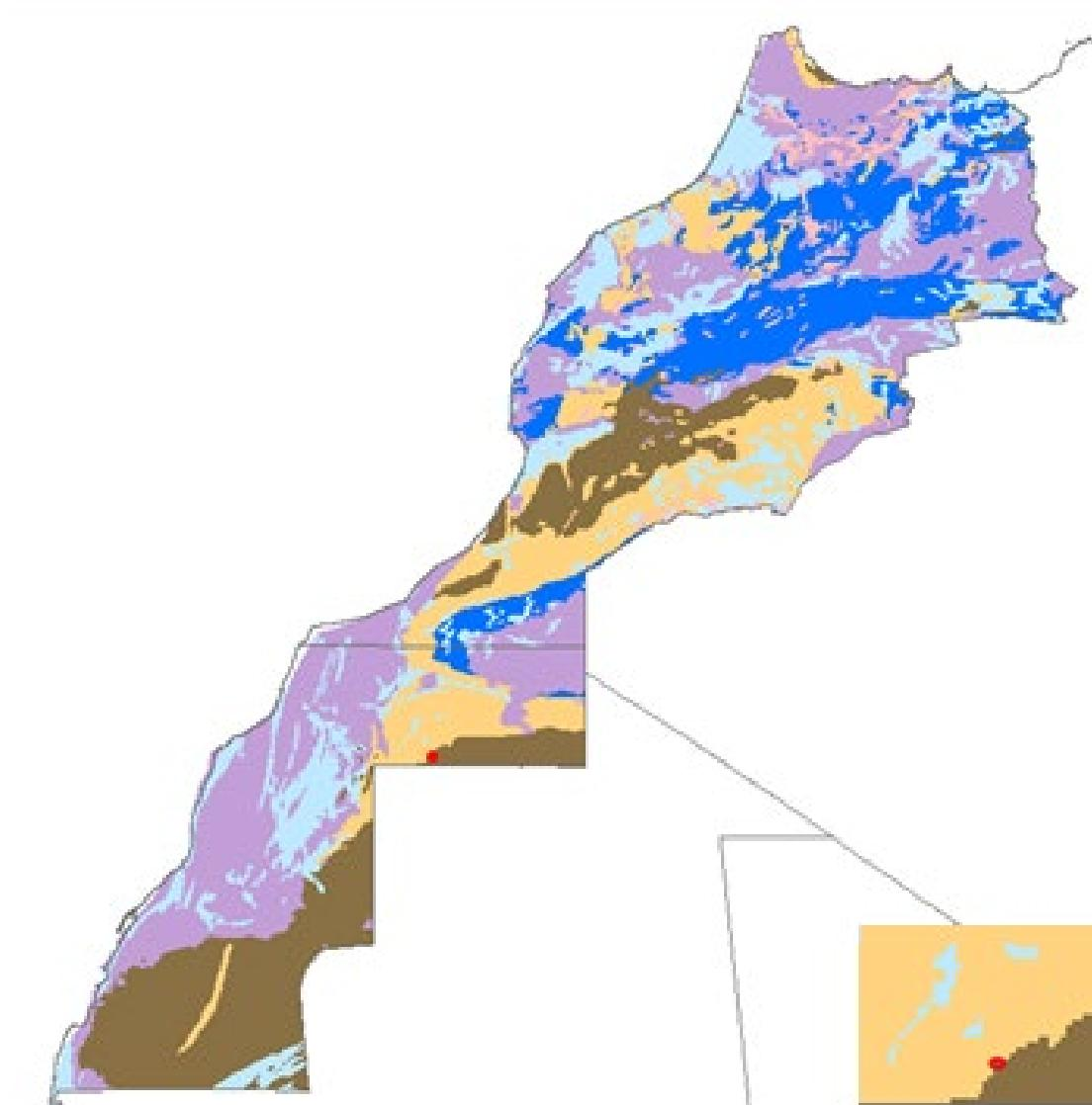
Figure 1: Aquifer type and productivity with location point
